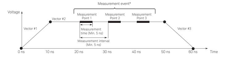
(\*) As well as the measurement event, the range change and trigger event can be specified in the vector.
